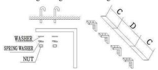
4.3.3 Set the mounting plate on the ceiling brackets and ensure safety & fixing (use the bolts attached to the ceiling brackets as Fig. Using the ceiling brackets to hang from the ceiling, the position of mounting plate can be adjusted in the limit of 100mm.
