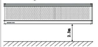
3.5 Don't allow gaps between the unit and the wall. When hanging it from the ceiling, purchase the extra ceiling brackets.
